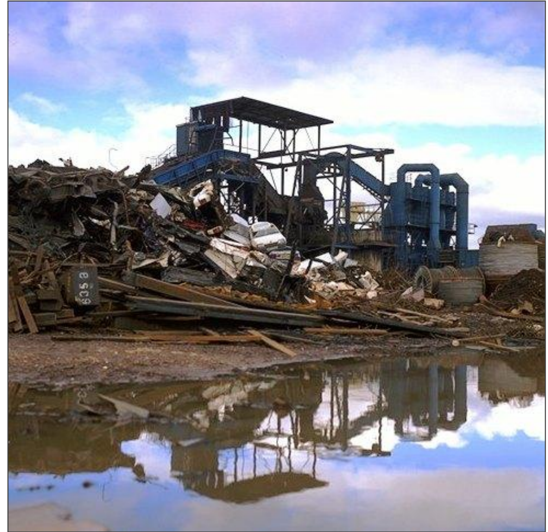
Poor surface water control & inappropriate surface
