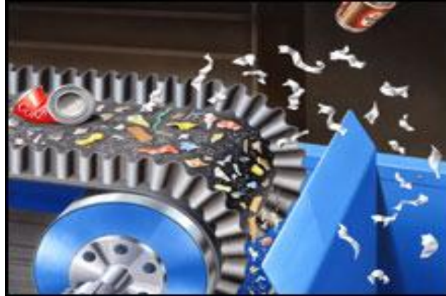
Eddy Current Separation (Aluminium)
