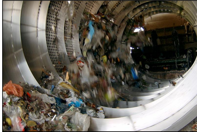
Trommel Screen (based on size)
